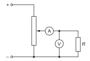
Which condition is necessary for an accurate value to be obtained for R?
