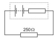
The current in the resistor is 40 mA for a time of 60 s. During this time 6.0 J of energy is lost in the internal resistance.
