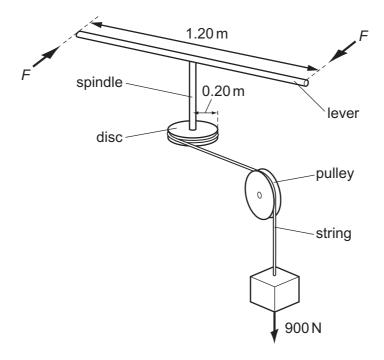
What is the minimum force *F*, applied to each end of the lever, that could lift the weight?
